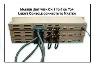
FIGURE 3 Stacking of MC4-H2 Units
